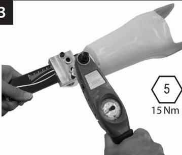
Tighten fitting clamp bolts to 15 Nm (check each screw at least twice).
