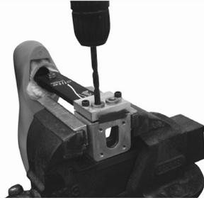
Drill two 8.1 diameter holes through drill bushes.
