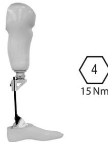
Fit socket to fitting clamp top housing and tighten pyramid screws (15 Nm). Refer to alignment page for initial setup.
