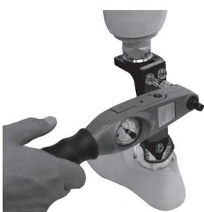
Cut blade using method shown previously before attaching top housing. Loctite (243) & tighten bolts (25 Nm). Re-apply cosmesis if applicable.
