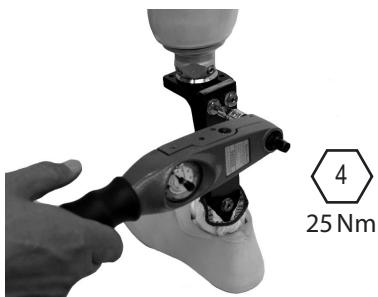
Loctite (243) & tighten (25 Nm) top housing bolts.
