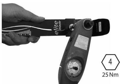
Attach blade to heel carrier. Loctite (243) & tighten bolt (25 Nm).
