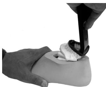
Remove blade from carrier/foot shell.
