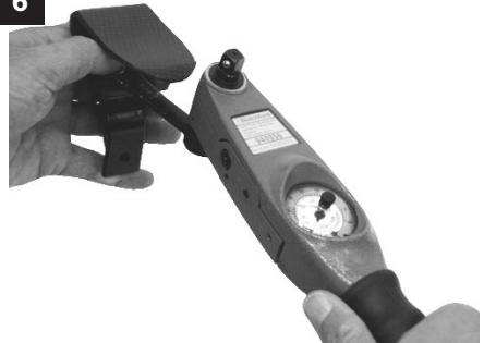
Fit new heel spring, Loctite (243) & tighten bolts (15 Nm). Use torque spanner attachment 940081
