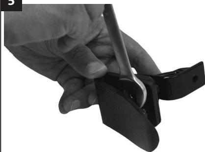
Remove heel spring from carrier.
